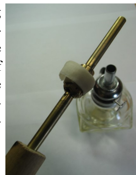
(Fig. 6) Removing initial dop with alcohol lamp. Stone and fingers protected by wet toweling on stone.
